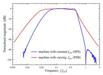
Figure 4: Typical AFE frequency characteristics.
