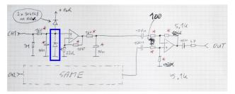
Figure 1: Original schematic of the high impedance amplifier built at BNL, with the marked error, very important for the future development.
