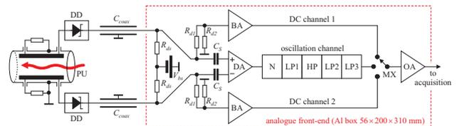
Figure 3: Block diagram of the 3D AFE with detectors.
