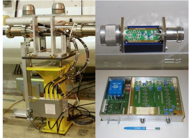
Figure 2: Typical 3D tunnel installation with the diode detector and the analogue front-end (LHC example).
