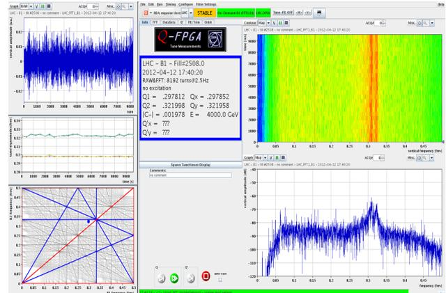
Figure 7: TuneViewer operated for the LHC.
