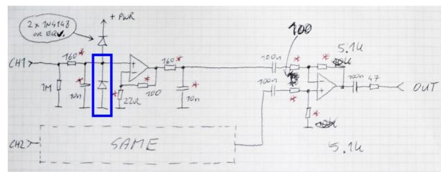
Figure 1: Original schematic of the high impedance amplifier built at BNL, with the marked error, very important for the future development.
