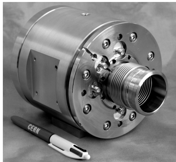
Figure 3: The IPU assembled. On the front there are four pick-up outputs and two calibration inputs.
