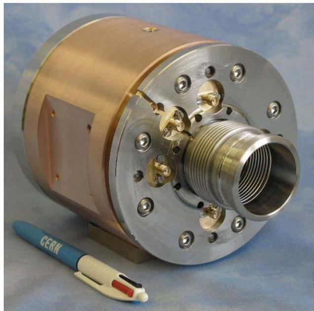
**Fig. 4.** The IPU of CTF3 assembled.
