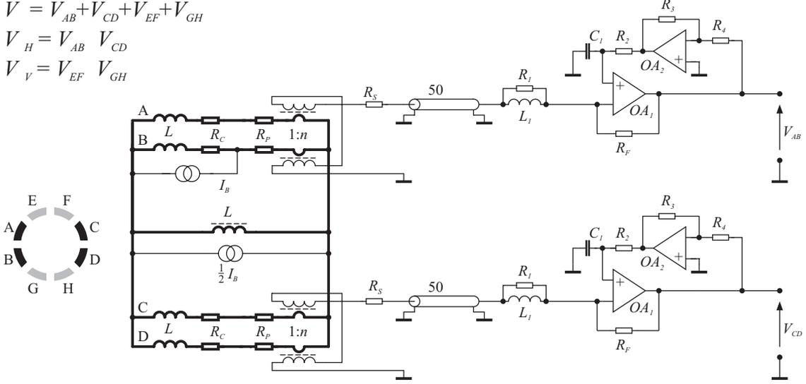
**Fig. 6.** An inductive pick-up model for one plane together with two channels of the transresistance amplifier.
