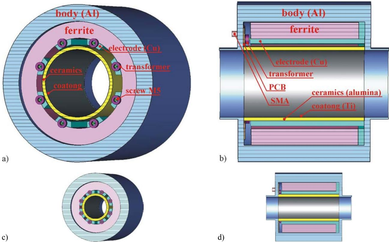
**Fig. 5.** Simplified cross-sections of the IPU being proposed (Fig. a and b) and the IPU of CTF3 (Fig. c and d). Scale about 1:4.
