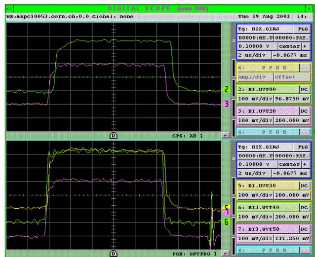
d) Cycle SFTPRO, 2  $\mu$ s/div, only calibration signals magnified.
